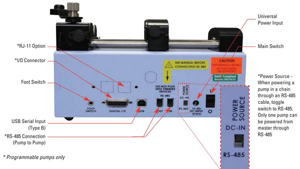
\*Power Source - When powering a pump in a chain through an RS-485 cable, toggle switch to RS-485. Only one pump can be powered from master through RS-485
